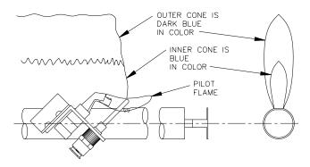
Figure 9.1: Standing Pilot and Main Burner Flame
